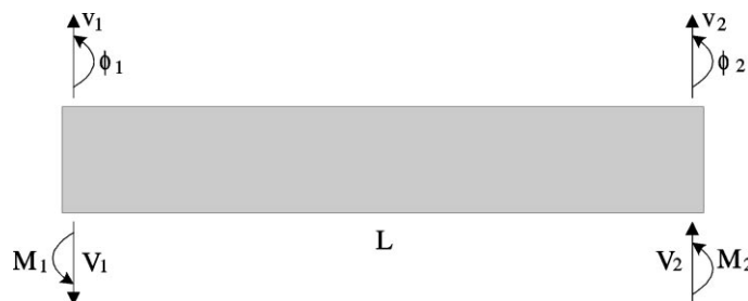
Fig. 2. Timoshenko beam with end loads and DOF.
